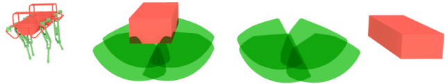
Fig. 2: The HyQ robot, and its simplified representation used to address \mathcal{P}_1 . The green shapes represent the reachable workspace of the effectors. The red shape is a bounding box that must stay collision-free at all times.
