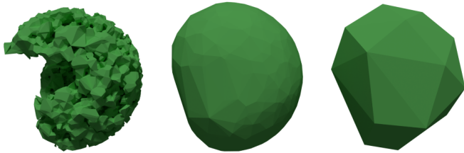
Fig. 15. Different approximations of the range of motion of the right arm of HRP-2. Left: non convex-hull, computed with the powercrust algorithm [39]. Middle: convex hull of the reachable workspace. Right: Simplified hull used in our experiments.
